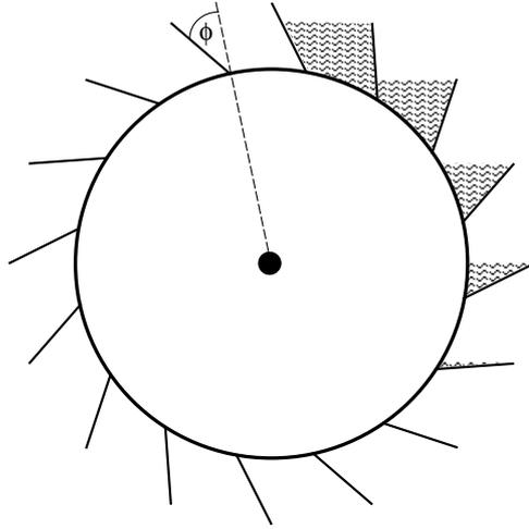
**Figure 2.** Overshot waterwheel with canted vanes (bucket separators). As the cant angle  $\phi$  increases, water is retained for longer, increasing torque.
