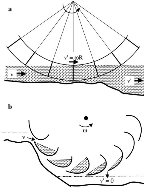
**Figure 4.** (a) Undershot waterwheel with radial vanes. The water flow approaching (receding from) the wheel has mean speed  $v$  ( $v'$ ). The wheel rotates at constant angular speed  $\bar{\omega} = v'/R$ . (b) Poncelet's modification: curved vanes that trap the water, releasing it only when the water has transferred most of its horizontal momentum. Achieving this requires a careful balancing of vane shape and water flow rate.
