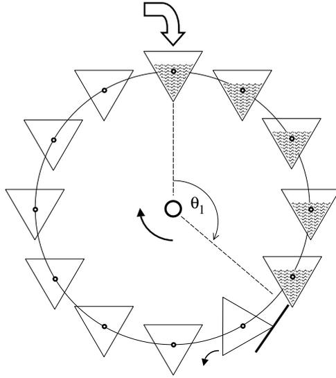
**Figure 1.** Idealized overshot waterwheel powered by gravitational potential energy (water head). Water drops vertically into buckets, and remains there until tipped out at angle  $\theta_1$ .
